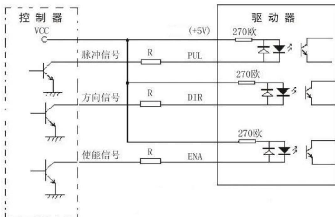
Fig 1. Input port circuit (Positive connection)
