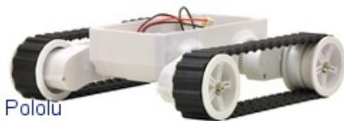
Dagu Rover 5 tracked chassis configured in its default, flattened position.
