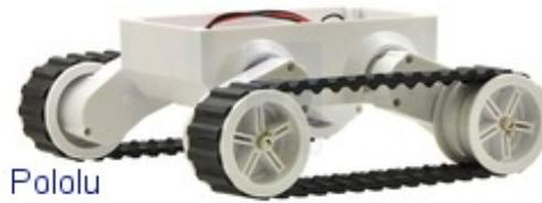
Dagu Rover 5 chassis configured in its maximally elevated position.
